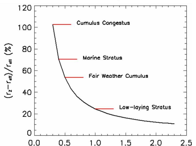
Figure 2. Percent error between effective radius,  $r_{\text{eff}}$  and the radar reflectivity based estimate of cloud drop size,  $r_Z$ , calculated based on the modified gamma drop-size distribution and cloud parameters tabulated in Ulaby *et al.* 1981 and the marine stratus distribution shape obtained from Vali *et al.* 1998.
