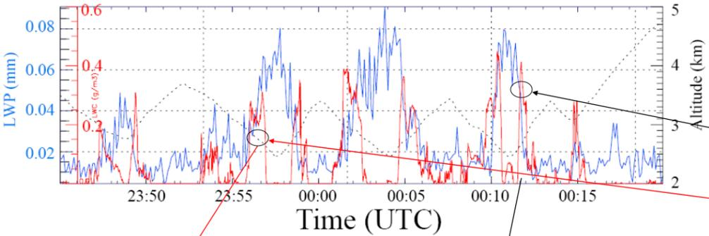
Figure 4. Aircraft in-situ probe measured liquid water content,  $w$ , (red) and GVR measured liquid water path (blue). Liquid water content ( $w$ ) was estimated from the GVR LWP data at two data segments as the aircraft changed altitude:
