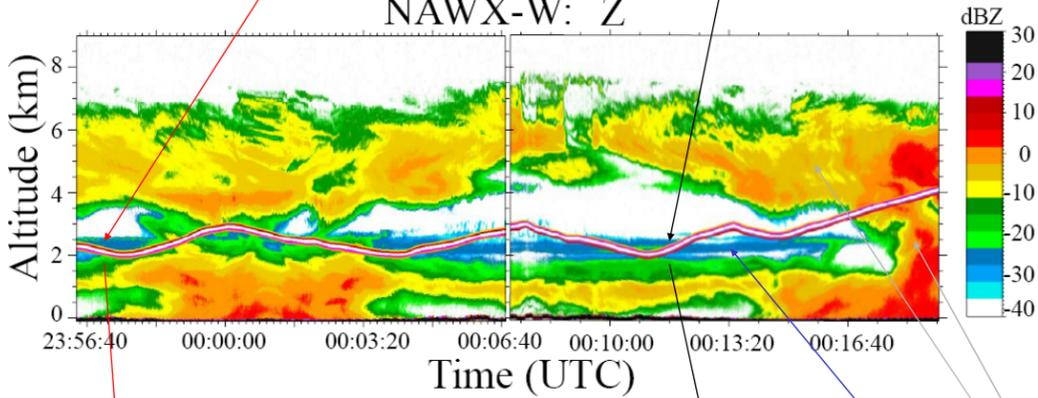
Figure 5. W-band radar reflectivity image. The nadir and zenith beams were combined to show clouds above and below the aircraft on an absolute altitude above sea level vs. UTC time scale. The aircraft flight path is indicated with a double red line in the image.
